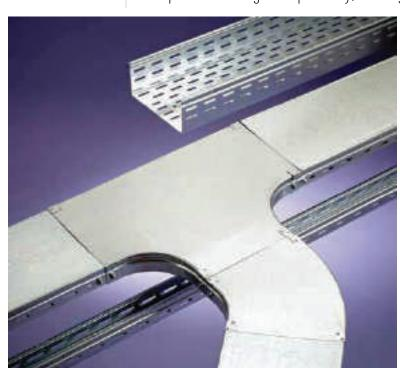
Ventilated Design All V-Trough straigh sections are ventilated to reduce cable bundle heating, and to keep mold and moisture from building up within the cab pathway.
