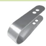
The RS1<sup>™</sup> rod stiffener is used with 1" Schedule 40 or Schedule 10 steel pipe and 3/8", 1/2" and 5/8" hanger rod. It snaps over the pipe and rod, and connects easily with a provided bolt and lock nut.
