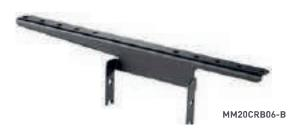
Mounts to the top side of the Mighty Mo rack channels or frames, providing mounting for wire cable tray to run parallel with the row of racks. Standard brackets position the bottom of the runway at 2" above the rack height and 6" high brackets position the bottom of the runway at 6" above the rack height.
