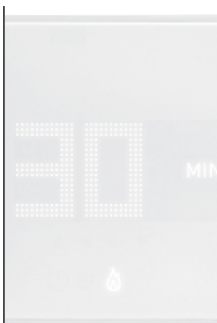
Select the duration (30, 60, or 90 minutes) and confirm. Heating is ON.
